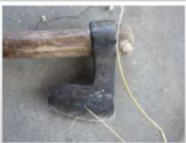
Bamboo culms are split by using a simple axe.
