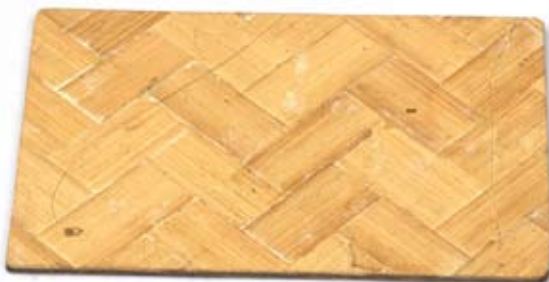
Two bamboo mats glued on plywood (from manufacturer)
