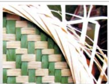
The craftsmen make three types of slivers. For mat weaving, banh is used. Banh is a thin and clean sliver with high flexibility.
