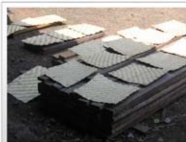
The mats are dried for 5 days; half a day in the sun and the rest of the time in the shadow.
