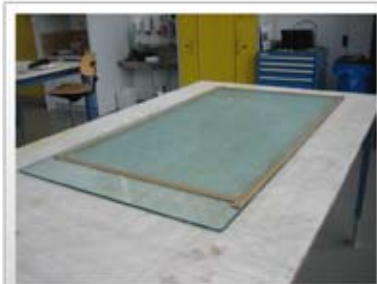
Vacuum bag sealing tape is fixed on a hardened glass plate which is used as mould.
