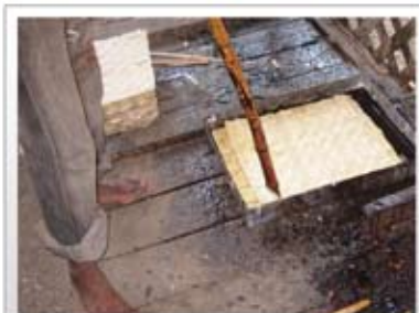
Mats are soaked for some minutes into the PF resin.
