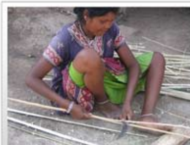
Sliver making is done with only a machete knife as tool. Tribal craftsmen are very skilled in this labour intensive work.
