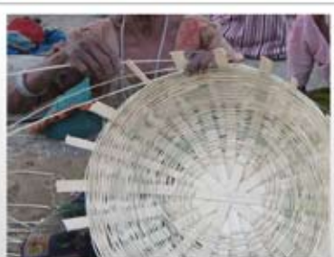
The third type of sliver is called hilly , which is used to fill the paat based construction of a basket.
