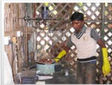
To make the resin, phenol, formaldehyde and sodiumhydroxide are mixed and heated up to 90/95 degrees Celsius. Sodiumhydroxide is used as catalyst.
