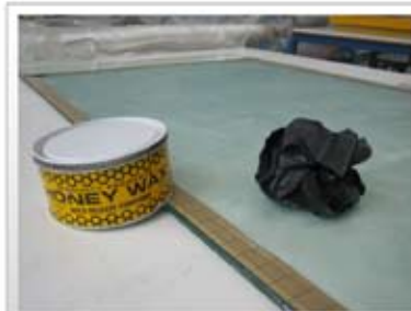
The mould is waxed with four layers of honey wax. The wax layers are air dried, after which they are rubbed off, leaving behind a smooth surface.
