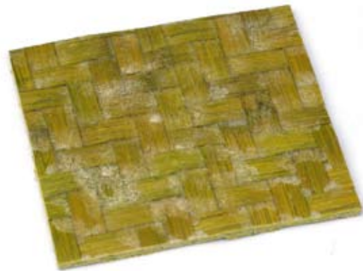
Two layers of mats glued together with foaming PU glue
