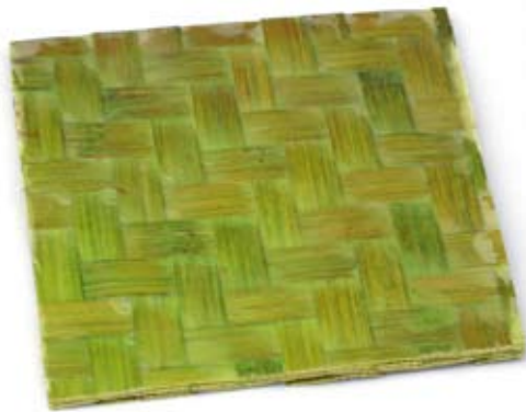
Two layers of mats glued together with white wood glue
