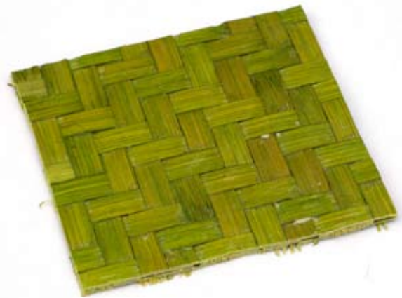
Two layers of mats glued together with epoxy
